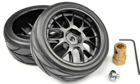
Fig. 11: Components to fix the driving wheels
