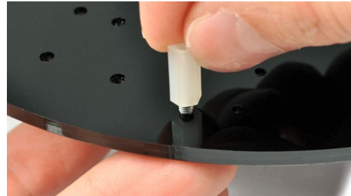
Fig. 57: Required parts to hold the PCB on the acrylic base
