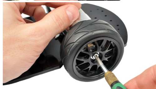
Fig. 12: Assembling the driving wheels
