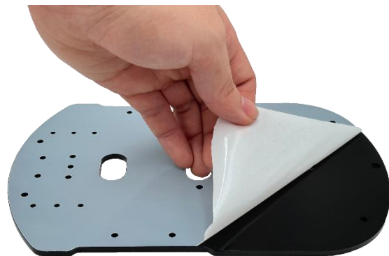
Fig. 6: Preparing the acrylic base
