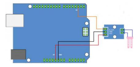
The water level sensor gives an analogue voltage corresponding to the water level present on the sensing element. If a larger proportion of the sensing elements are exposed to water, the output voltage will increase.
