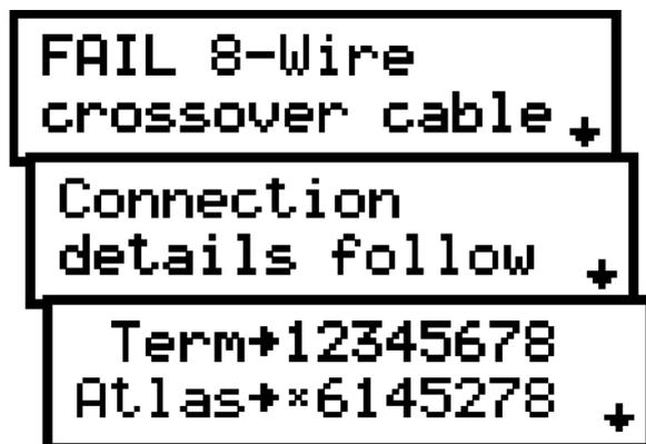
In this example, the closest cable type match is an 8-wire crossover cable. Pressing the **scroll-off** button to view the next pages reveals the nature of the fault.
