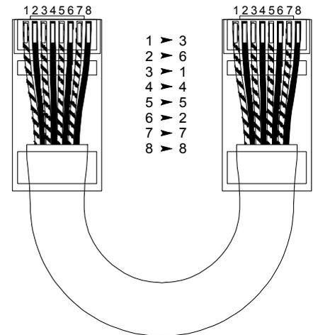
Please note, there are actually a number of wiring configurations that can be used to produce a crossover cable. The cable connection pattern shown above is the most common. However, the *Atlas IT* will recognise all variations.
