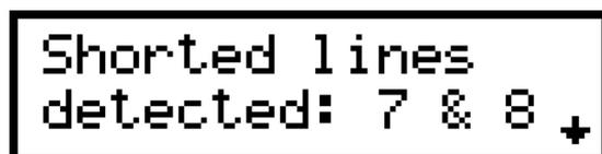
This message means the *Atlas IT* has detected a short circuit between the two lines, 7 & 8. These line numbers are as
