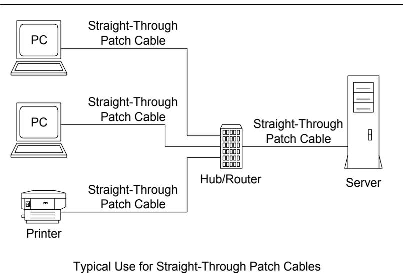
These are generally used for connecting computers to hubs (routers or switches) or simply between a PC and a wall socket (which eventually connects to a hub).
