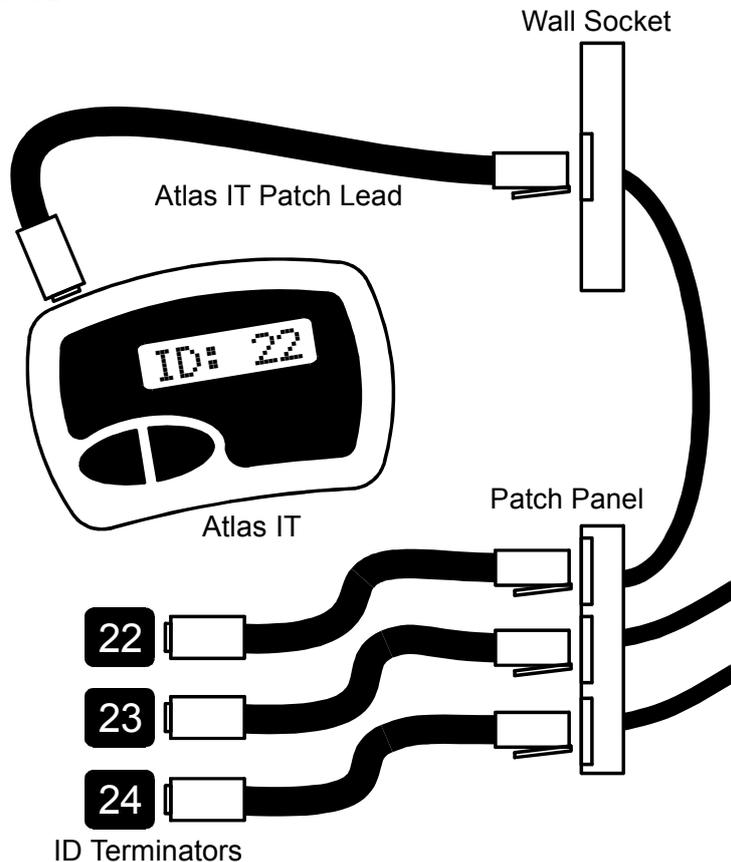
These special terminators can be used in exactly the same way as the standard (non-identified) terminators. They are automatically recognised by the *Atlas IT* and the identity number is displayed along with the cable analysis results.
