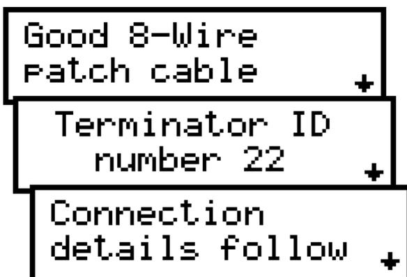
Up to 24 Identified Terminators are available, allowing for the rapid testing, and identification of large numbers of network cables or sockets.
