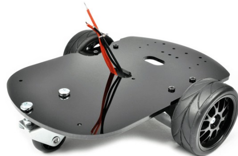
Fig. 14: Assembling the caster wheel and adjusting of the robot inclination
