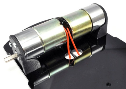
Fig. 10: Passing the motors wires through the acrylic base
