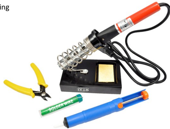
Fig. 15: Required material for electronics assembly
